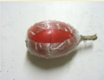
Figure 5: Fiber tape for longitudinal reinforcement.
