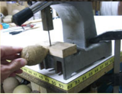
Figure 9: Punching crossmatch hole after case dries.
