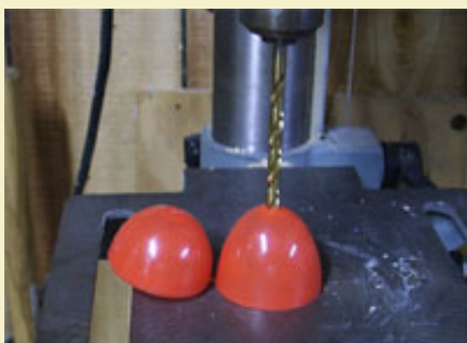
Figure 1: Drilling 7/32" time fuse hole.
