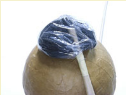
Figure 11: 120g lift bag positioned over cross-matched time fuse.
