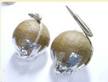
Figure 12: Foil tape used to secure and protect the lift charge.
