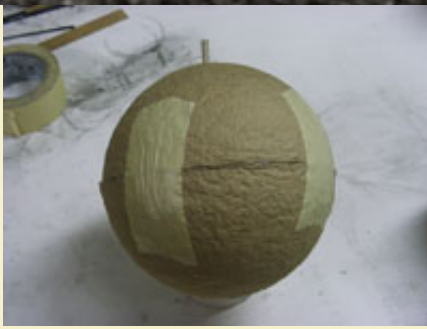
Figure 9: Halves brought together by tapping with a stick, then held with tape.
