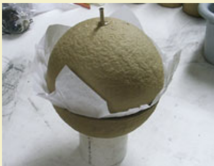
Figure 8: Sheet of tissue used to prevent spills when one shell half is inverted onto the other.
