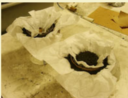
Figure 11: Tissue paper liner placed over inner petal stars and filled with burst charge.
