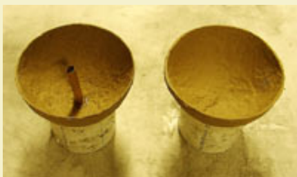
Figure 5: Center tube hot glued over time fuse.
