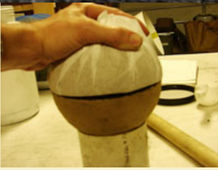
Figure 14: Closing the gap by tapping with wooden stick.
