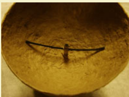
Figure 4: Cross matched time fuse inserted through bottom of hemisphere.
