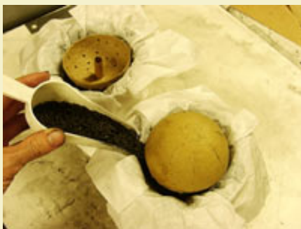
Figure 9: Pouring break charge around inner hemis.
