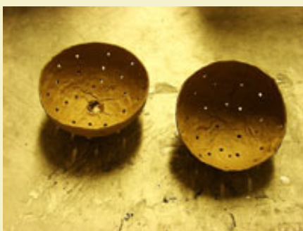
Figure 8: Inner hemispheres punched with holes to help fire transfer.
