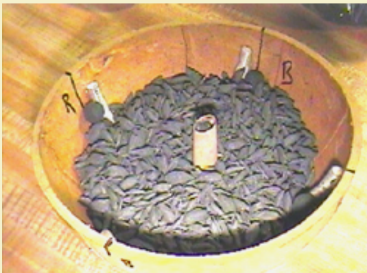
Figure 12: Partial burst charge loaded on top of ring stars.
