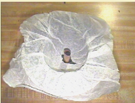
Figure 16: The former is removed and the cavity is ready for stars.
