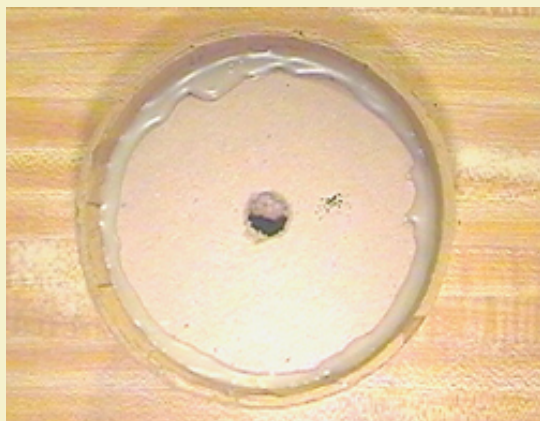
Figure 2: A 3" paper hemi to be used as a cavity former is reinforced with a cardboard disk to prevent warping.
