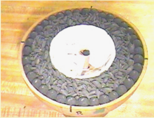
Figure 14: Burst charge and ring stars loaded in around the cavity former.
