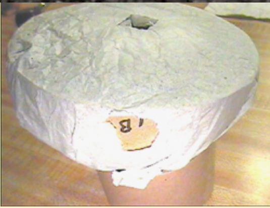
Figure 20: Piece of tissue placed over one shell half prior to inverting it onto the other half.
