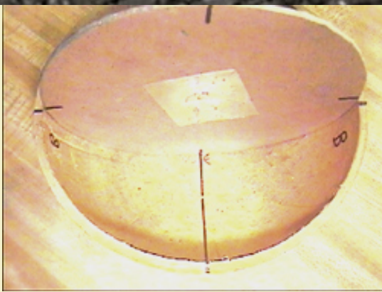
Figure 7: Marking the second, intersecting ring guideline.
