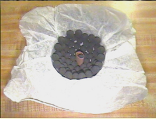
Figure 17: Loading stars into the 3" cavity to form the "nucleus" of the atom pattern.
