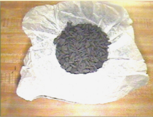
Figure 18: Remainder of space is filled with burst charge.
