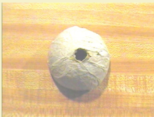
Figure 3: The cavity former is covered with
