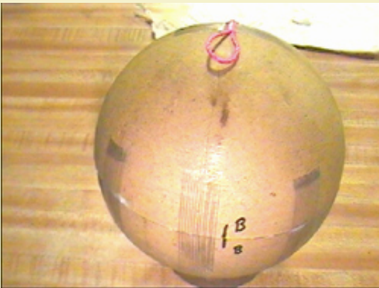
Figure 21: The shell seam is held together with pieces of fiber tape after closing the two halves together.
