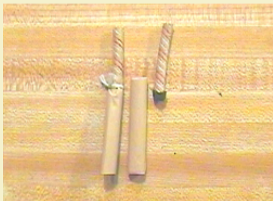
Figure 1: Preparing primed time fuse with an extension pipette.
