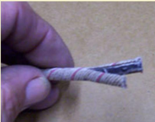
Figure 5: Split fuse after cutting.
