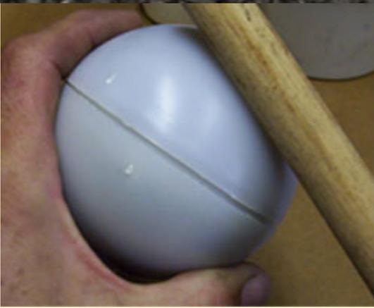
Figure 15: Closing the shell by tapping with a rod.
