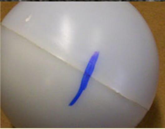
Figure 3: Marking the best aligned position before assembly.
