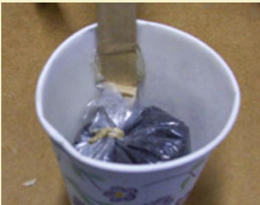
Figure 23: Lift assembly loaded into a paper cup.
