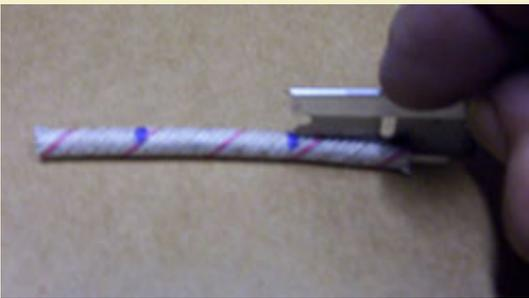
Figure 4: Splitting the flash bag end of the time fuse.
