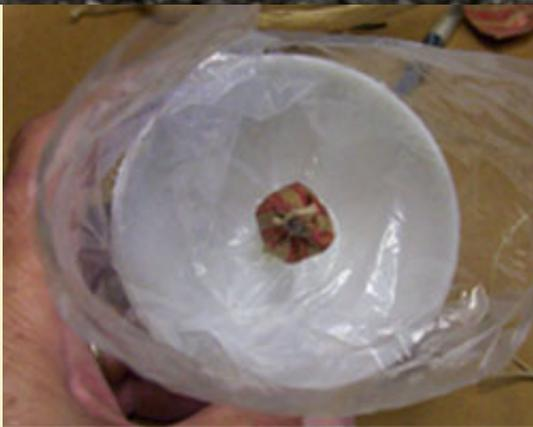
Figure 12: Plastic bag inserted prior to loading.
