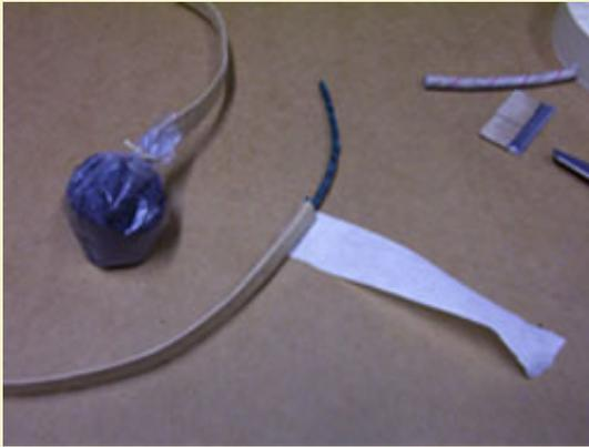
Figure 21: Securing visco into leader using masking tape.
