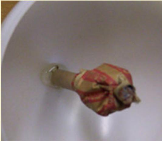
Figure 10: Fuse assembly glued into the shell.
