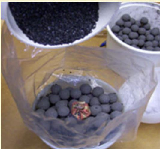
Figure 13: Adding 4FA after half the stars are loaded.
