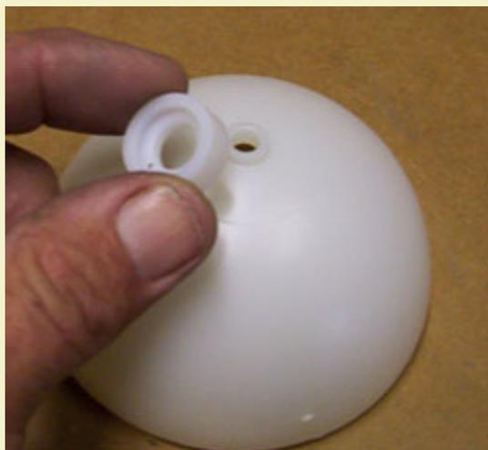
Figure 2: Gluing on the time fuse ring.
