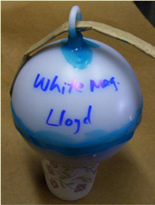
Figure 27: Finished shell ready to fire.
