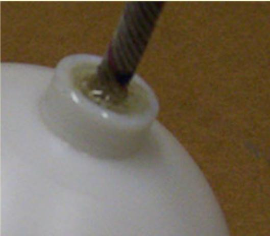
Figure 16: Close up showing glue seal around time fuse.
