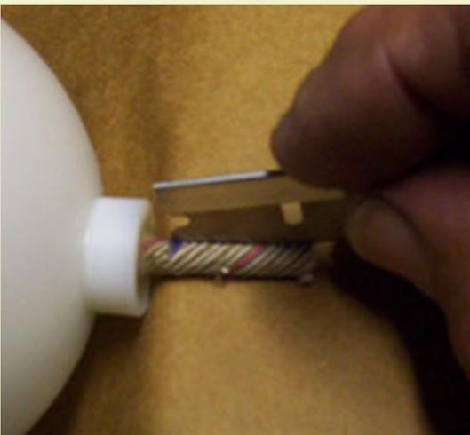
Figure 17: Splitting the outside end of the time fuse.
