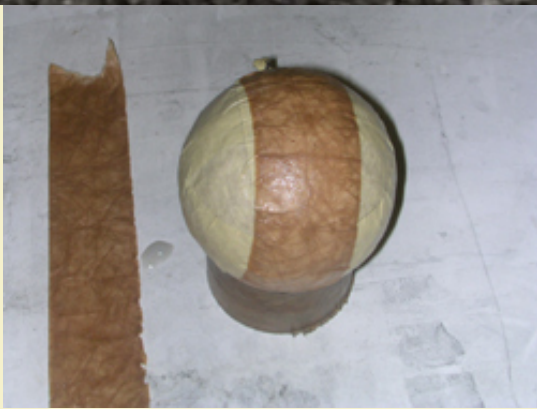
Figure 16: The paste pattern starts with one full wrap around the shells circumference.
