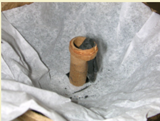
Figure 13: Securing the passfire match into the shell pipette with twine.
