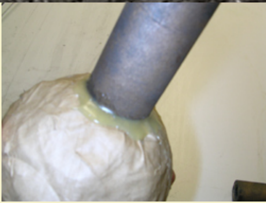
Figure 19: Attaching the dried header shell to the engine using hot glue.
