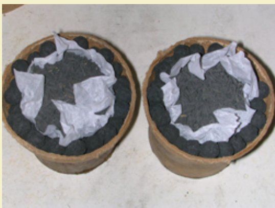
Figure 14: The shell hemis loaded and ready to close.
