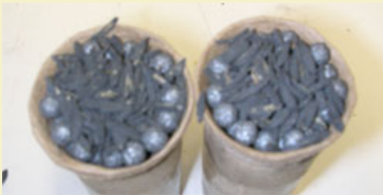
Figure 6: Burst charge of 7:1 KP on rice hulls.
