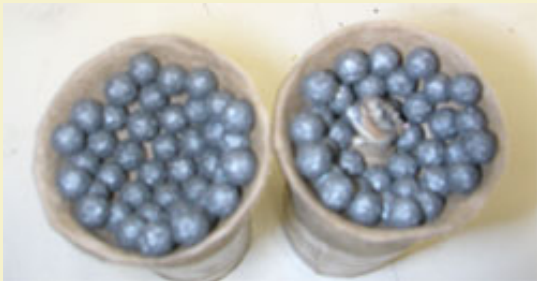
Figure 5: Stars stacked around sides in single layer.
