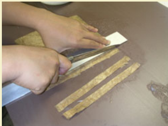
Figure 12: Slicing off 9/16" wide strips with a sharp knife.
