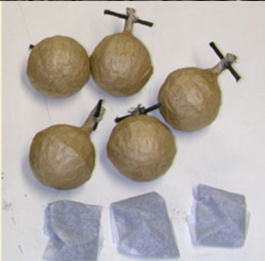
Figure 15: Finished shells with 5g lift bags.
