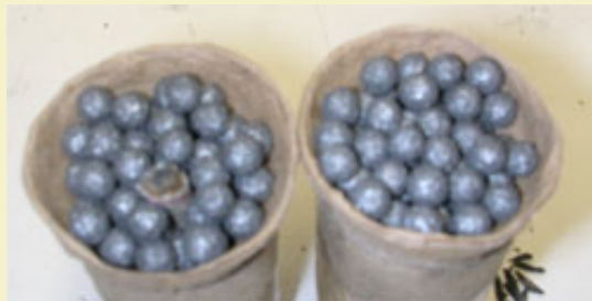
Figure 2: Both hemis filled with 7/32" dia. stars.
