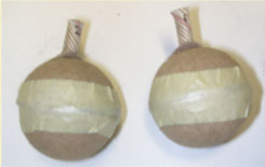
Figure 9: Hemis held together with a band of 1/2" masking tape.
