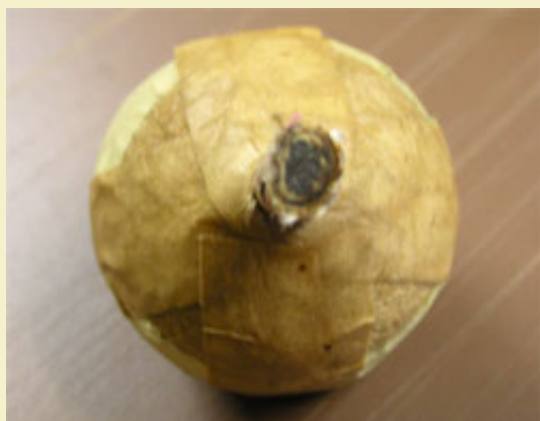
Figure 13: First two pasted strips meeting at the time fuse.
