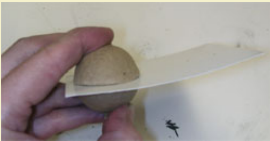
Figure 8: Sliding out a sheet of poster board used to reduce spilling when joining hemis.
