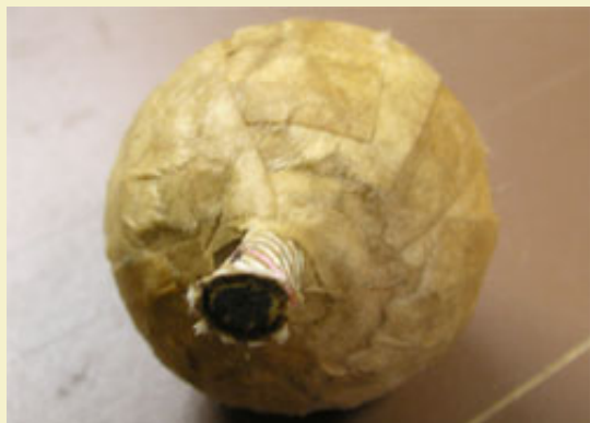
Figure 14: Remaining four quadrants pasted with overlapping strips.
