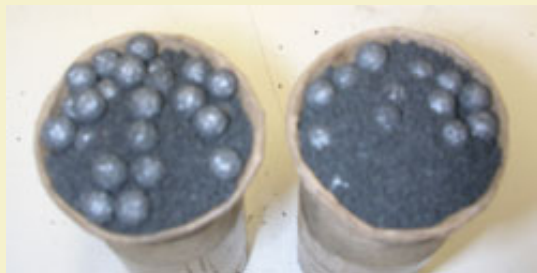
Figure 3: Burst charge of 1/2 TSP 2Fg in each hemi.
