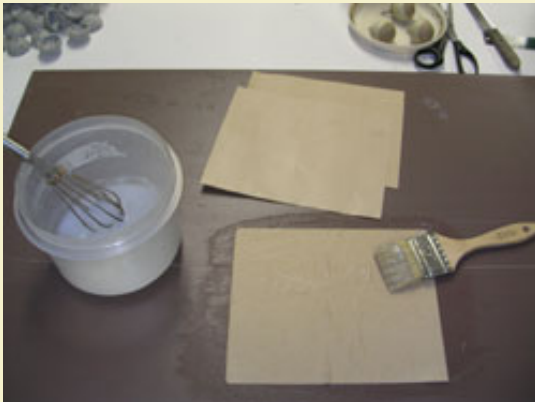
Figure 10: Pasting a 4-sheet stack of 30lb virgin kraft.
