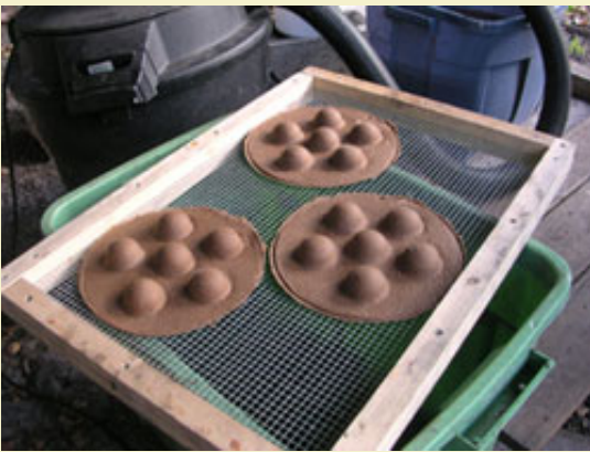
Figure 11: Output of the mold operation placed on drying screens.
