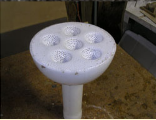
Figure 10: The finished 6 piece 1-1/2" vacuum form mold.
