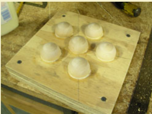
Figure 2: Removing hole centers on male side of mold.
