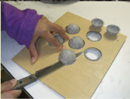
Figure 13: Using a saw or knife to easily trim hemis from mold.
