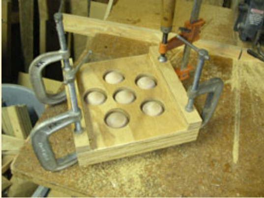
Figure 4: Gluing standoff feet to bottom of female mold.
