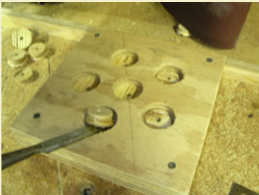
Figure 2: Removing hole centers on male side of mold.
