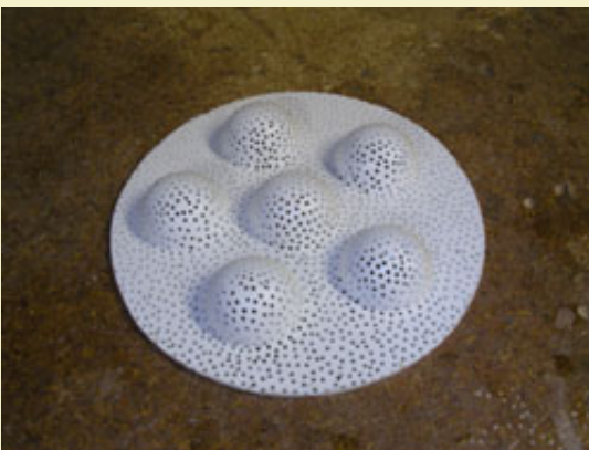
Figure 9: A PVC mold plate after drilling and trimming to fit an 8" shell casing.
