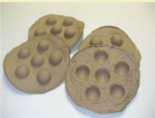
Figure 12: Paper molds dried and ready for separation.
