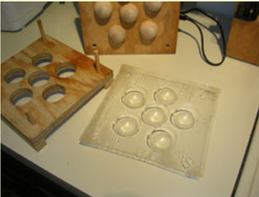
Figure 8: An acrylic mold removed after mold has completely cooled.
