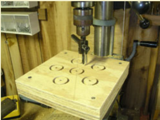
Figure 1: Drilling out large holes with an adjustable hole cutter.
