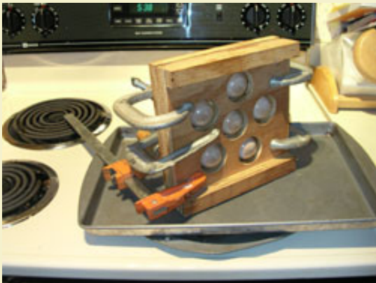
Figure 6: Clamping mold halves firmly together after coming out of the oven.
