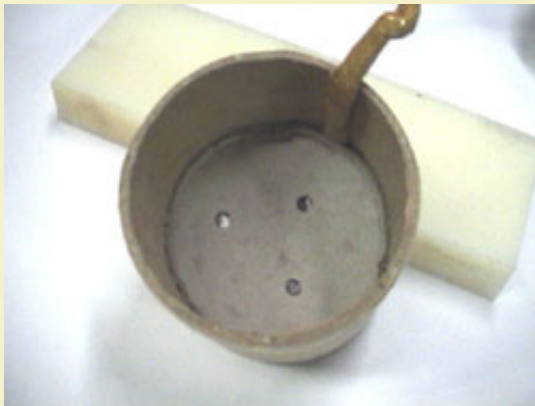
Figure 4: Perforated "piston" disk above the lift charge.
