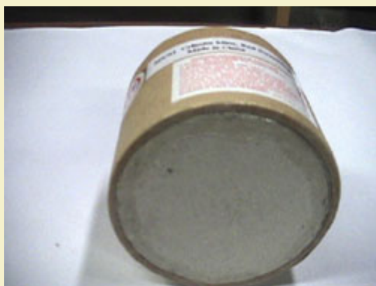
Figure 2: Bottom of mine sealed with a cardboard plug.
