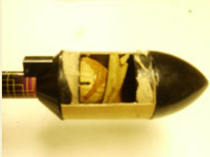
Figure 2: Heading contains over 50% empty space.
