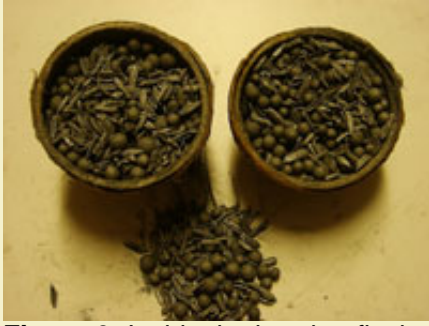
Figure 6: Inside the header, flash coated rice hulls with core-less colored round stars.
