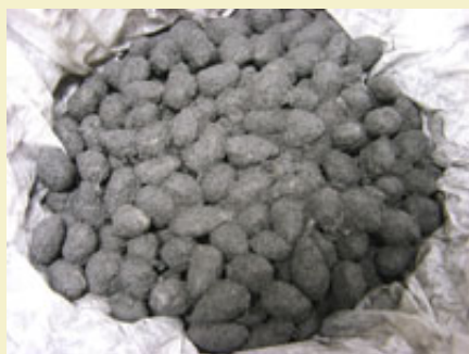
Figure 2: Burst charge of KP on cotton seed loaded into planet stars.
