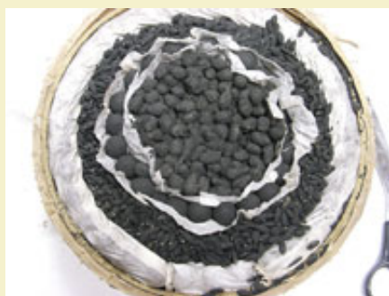
Figure 1: Half containing ring stars and inner planet stars. Note the layers of tissue used to hold the planet stars.
