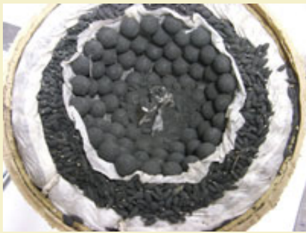
Figure 3: 1/2" dia planet stars set into 4-1/4" dia pressed cavity.
