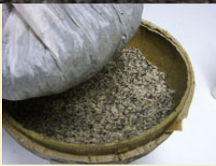
Figure 3: Inert filler used at both ends of the hemispheres to reduce the volume of burst charge.
