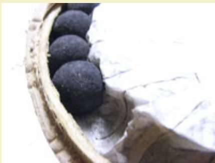
Figure 2: Stars are wedged tightly into a tissue paper trough.
