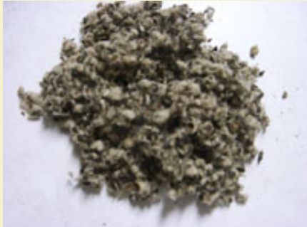
Figure 5: Closeup of filler reveals some sort of ground cotton seed material.
