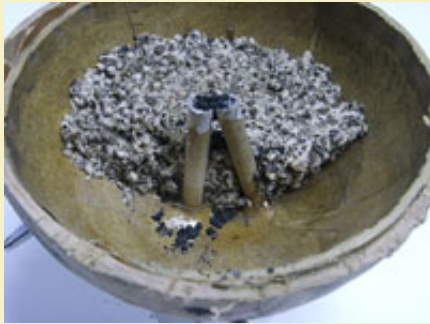
Figure 4: Thickness of filler was measured to be 1-1/4" deep at center.
