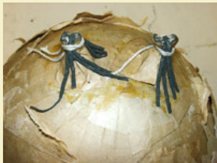
Figure 2: Time fuse crossmatched with split & tie method.
