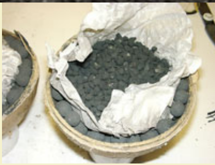
Figure 3: Black powder on cotton seed as the break charge.
