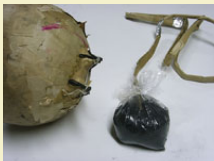
Figure 1: The plastic bag of lift with time fuse tied in was pasted onto the shell.
