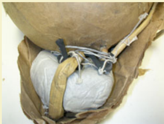
Figure 2: Leader tied to time fuse, with separate leader going into lift bag.
