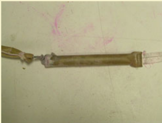
Figure 17: Close-up of the red flare, which burns for 27 seconds following a 6 second pre-ignition delay.
