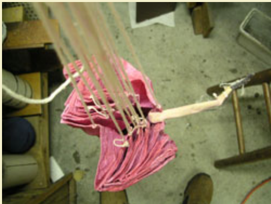
Figure 14: Piped Chinese fuse leading inside the chute where the flare is located.
