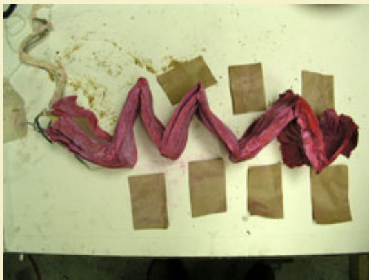
Figure 12: Accordion style folding of chute, with slips of paper placed between the folds.
