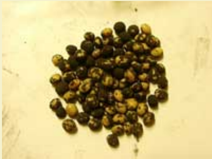
Figure 6: A mixture of inert, meal coated beans are mixed with 2FA and 3FA for the burst.
