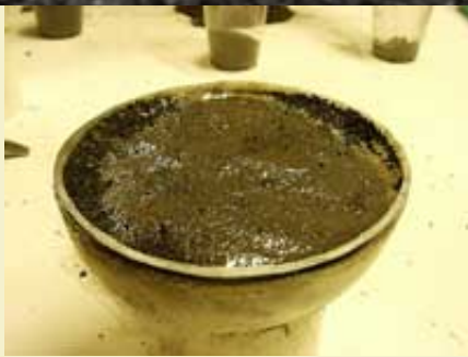
Figure 5: The other hemi is covered with thin, vented plastic prior to closing.
