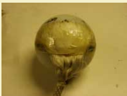
Figure 2: Fiber tape holds frayed rope end to shell casing.
