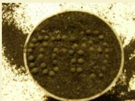
Figure 4: The elephant pattern embedded in 4FA BP within the time-fuse hemi.
