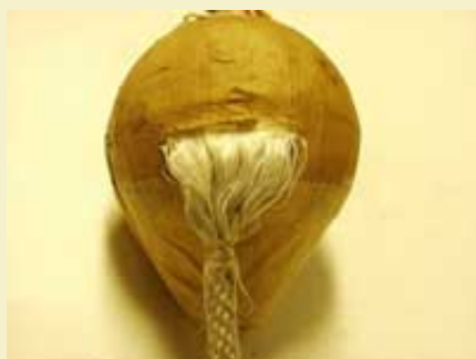
Figure 1: Rope attached at equator to stabilize pattern orientation.
