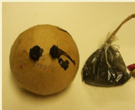
Figure 1: Double time fuse with plastic bag for lift charge.
