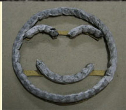
Figure 5: Pattern held solidly together by both cardboard backing and tissue wrap around stars.
