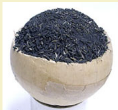
Figure 3: Densely packed rice hull burst charge.
