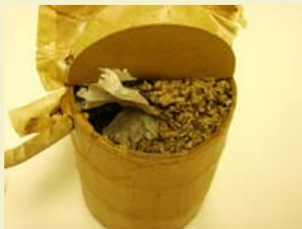
Figure 2: Thin bottom disk peeled open to reveal lift charge and filler.
