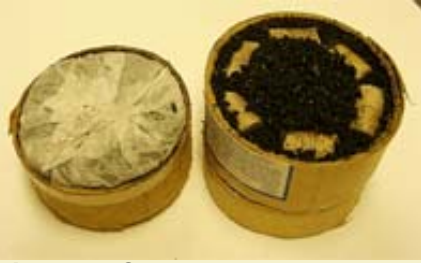
Figure 4: Shell loaded as typical for ball shells.
