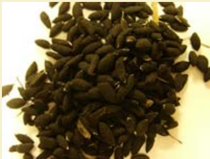
Figure 6: Closeup of KP burst charge.
