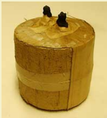
Figure 3: Stripped away paste layer shows cylindrical strawboard
