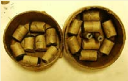
Figure 5: Placement of crossettes in second layers.
