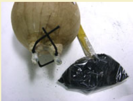
Figure 1: Bagged lift with plastic coated leader.
