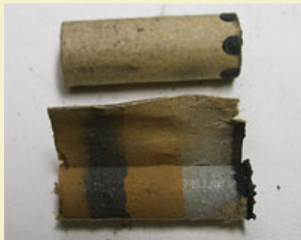
Figure 8: Insert charge from left to right: clay, flash, clay, white strobe and prime.
