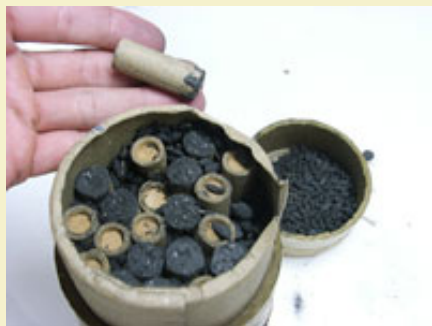
Figure 7: Inserts completely fill bottom compartment, with prime end randomly oriented.
