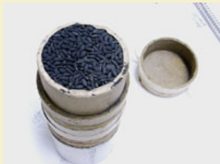
Figure 6: Top cap removed reveals KP burst charge packed around inserts.
