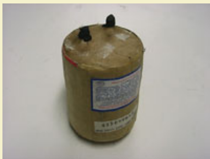
Figure 2: Strip pasted can with slurry primed, dual piped time fuse.
