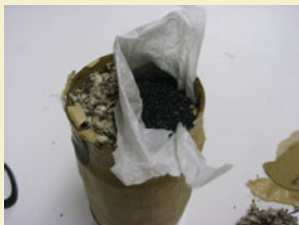
Figure 1: Lift charge contained in paper liner surrounded by ground cotton seed.
