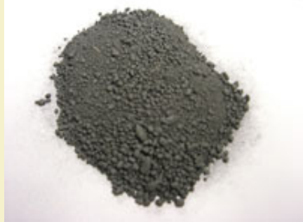
Figure 5: Dark, granulated flash of moderate burning speed used to break the star portion of the shell.
