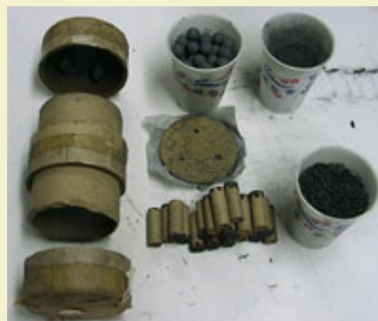
Figure 3: Disassembled shell with all components.
