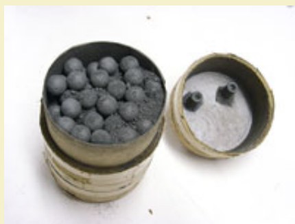
Figure 4: Bottom cap removed (time fuse end) to reveal star compartment with granulated flash break.
