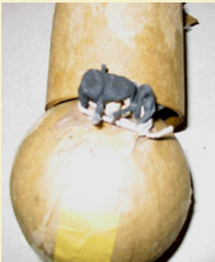
Figure 4: Thick prime on upper shell.
