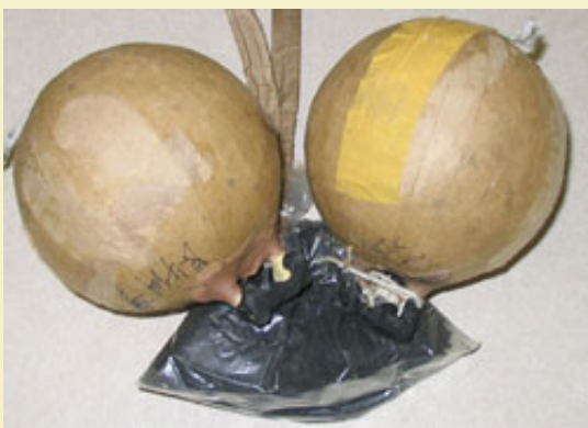
Figure 5: Both shells shown with plastic lift bag.
