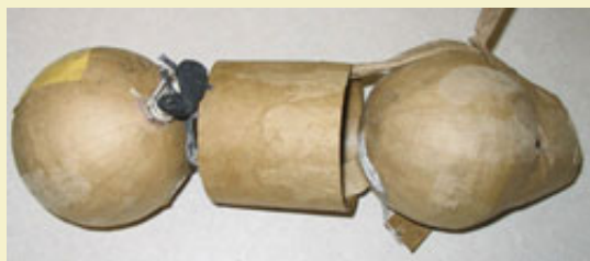
Figure 2: Quickmatch passfire used to ignite 2nd shell.
