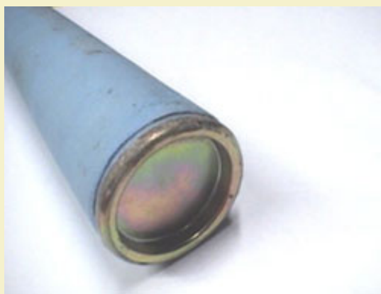
Figure 2: Spiral tube plugged with metal end cap at bottom.
