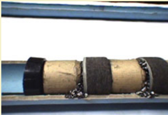
Figure 4: Closeup of crossette, lift and delay wadding for each shot.
