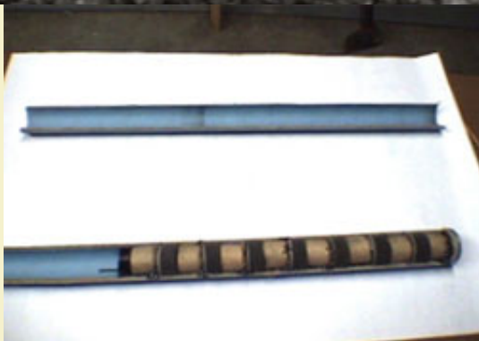
Figure 3: Cross section showing arrangement of eight shots.
