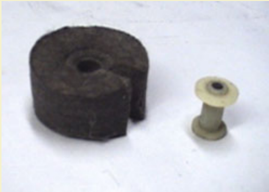
Figure 7: The felt wadding and timer spool used to create the delay between shots.
