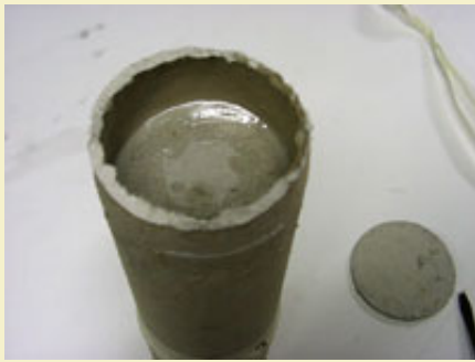
Figure 3: Triple disk inner plug held in place with lots of white glue.
