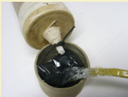
Figure 4: Bottom fused with plastic lift bag. Note the amount of glued string wrapped around the time fuse base.
