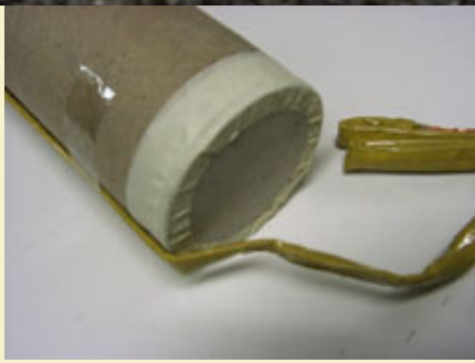
Figure 2: Outer disk held on with masking tape.
