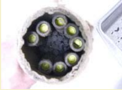
Figure 6: Fused end cap removed, looking down at the tourbillions. Note the yellow plastic end plugs.
