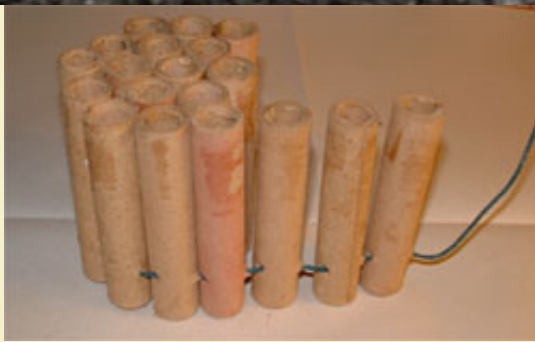
Figure 3: Shot tubes threaded onto long strand of Visco.
