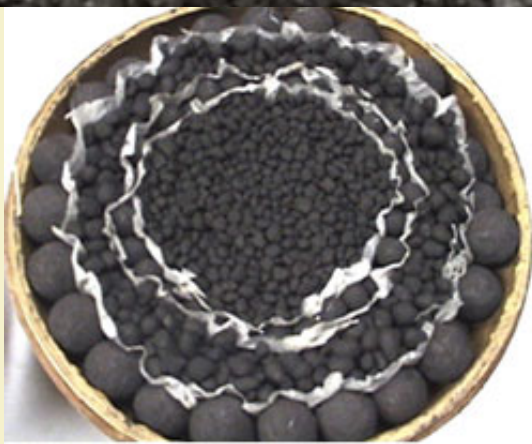
Figure 3: Tissue paper cut away to show separate petals and break charges.
