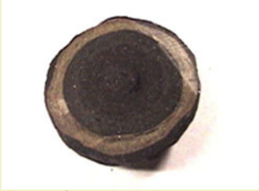
Figure 6: Cross section of 1" outer petal star reveals layers of color changing composition.
