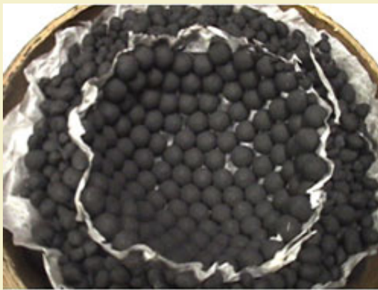
Figure 4: Inner break charge removed to reveal inner petal stars
