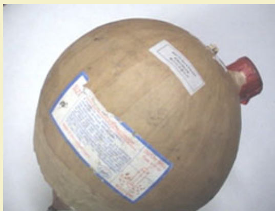
Figure 1: Outer casing with rising comet.
