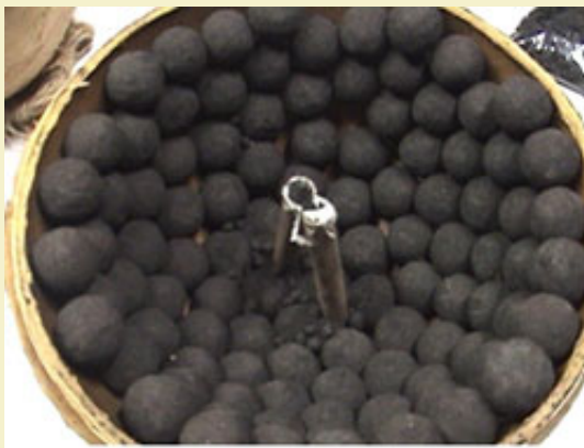
Figure 5: Outer break charge removed to reveal passfire tubes in lower hemisphere.
