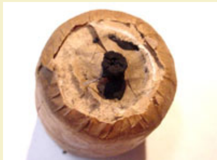
Figure 4: Slurry primed chinese fuse.
