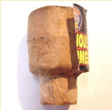
Figure 2: Lift cup pasted onto shell with a turn of light weight kraft.
