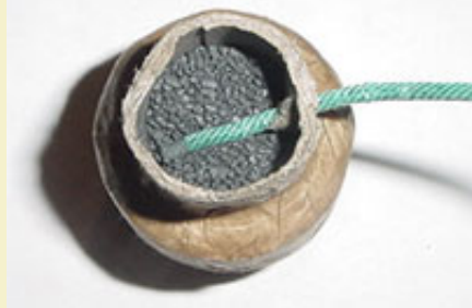
Figure 3: Lift cup filled with 3.9g of 2Fg.
