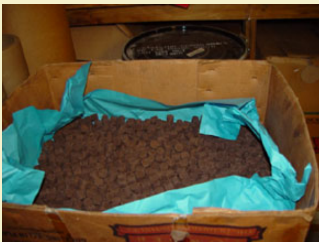
A box of 3/4" stars pumped 70 at a time using a hydraulic press.
