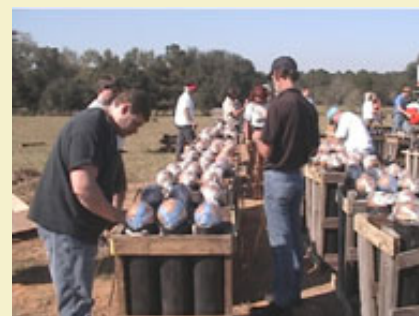
Over 100 6" paper ball shells being loaded into racks.
