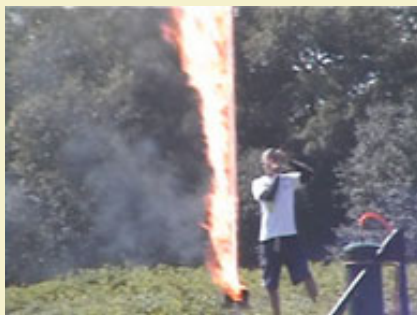
Compressed CO2 forces liquid kerosene through a nozzle, past a pilot flame and then almost 100 feet into the air.
