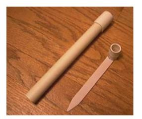
First, a reinforcing sleeve is made from an 8.5 inch length of 3/4 inch CPVC. This pipe has an inside diameter of 11/16 inches even though its name implies that it should be 3/4 inches. A coupler is glued to one end to act as a crude funnel for adding the sparkler comp. Now take a coupler for 1/2 inch CPVC and hot glue it to a handle stick as in the picture. This is your high tech scoop.
