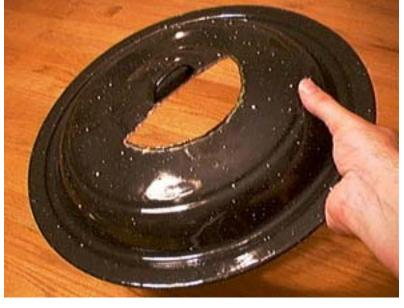
A lid for your "oven" must be fashioned with a hole in it where the hot gases can exit. The idea is to create a draft of hot gases from the bottom of the oven to the top. If you use this kind of pot, it's a good idea to cut the hole with minimal damage to the surrounding porcelain.
