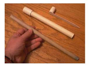
The next step is to make a simple rammer from a 12 inch length of 5/8 inch diameter dowel. Sand it to remove any rough edges and imperfections and seal it with some kind of sealer. If your not a perfectionist, you don't even need to bother with the sanding and sealing. This ram will be quite loose in the tube so precision is not a major concern.
