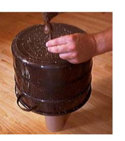
Next. the holes in the bottom of the pot are made. I placed a length of 3 inch paper mortar tube with its face against the inside bottom of the pot, beneath the site of each hole. This gives firm support to the bottom surface which avoids cracking the porcelain while the holes are formed. A sharp blow with a hammer on a center punch creates a hole
