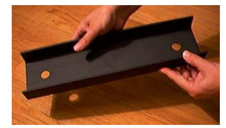
These first pictures show some of the major component parts of the press. This is one of two pieces of 4 inch wide channel. They are 16 inches long and are used at the top and bottom of the press. They are useful for mounting eye bolts and the blast shield as well as providing a
