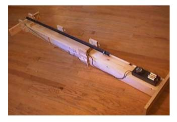
The stop thread can be secured by an identical arrangement at either 45 cm or 100 cm from the start thread. The wood block which holds the stop microswitch can easily be moved by removing the two screws which secure it to the platform. This angle shows that the micro-switch has a small restraining block glued to it which limits the travel of the switch actuator. This shortens the time for the switch to register the change in state when the thread has been severed by the flame front.
