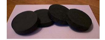
has been designed so that the finished press cake has the desired density of 1.7 grams/cc.
