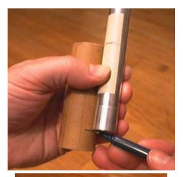
Next, remove the rammer and hold it against the outside of the tube with the mark you just made even with the top of the tube. Make a mark on the body tube at the bottom of the rammer. This mark should now indicate where the top of the nozzle is inside the tube.
