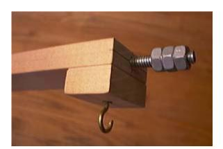
The ends of the beam are constructed as shown to lower the swivel point of the weight pans. This is done by simply gluing another block of poplar to the bottom of the beam at each end. Next, the hooks are added from which the weight pans are hung. Finally, pieces of threaded rod are screwed into the ends of the beam and 2 or 3 nuts are screwed onto the rods. These are used as adjustment weights to cancel any asymmetries in the balance beam.
