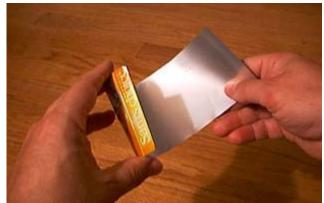
Now cut down the length of the can. When finished you will have a curly rectangle of aluminum about 4 inches wide by 8 inches long. From this rectangle you can cut two trapezoidal shapes with a long side of about 4 inches and a short side of about 2.5 to 3 inches. You can tailor the short side to the size of tube you will be filling with the funnel.
