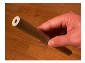
There are only two basic tools in the tooling set for fountains. One is the nozzle former, or spindle, and the other is the rammer, or "drift" if you want to use a nice buzz-word. The first step in making this tooling is to drill a hole into the end of a dowel to serve as the rammer. The hole is the same diameter as the spindle which, in this case, is 1/4 inch. The dowel is the same
