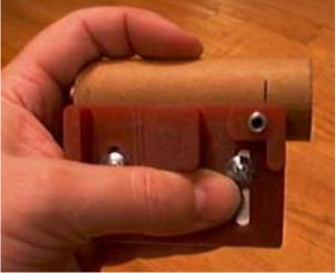
Now the tube is held in the drilling jig, as shown. The guide hole should be located so that the side vent hole will be drilled just above the nozzle. In case you haven't figured it out, you'll probably have to remove the tube from the spindle base to drill the side vent hole.
