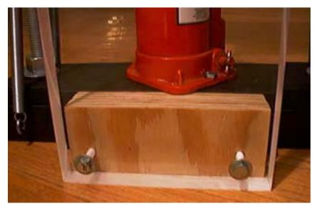
This picture shows the attachment of the blast shield to the base channel. You can also see the bolt which secures the base of the hydraulic jack to the base of the press frame.
