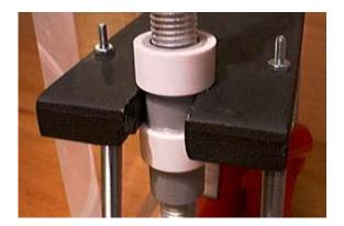
This idea comes to you from Rich Weaver. I liked it so well, I made the modifications to my own press. The concept is to add protective sleeves around the threaded rods to prevent the press deck from scraping against them as the deck is raised and lowered. I made the sleeves from 3 inch lengths of 3/4 inch PVC conduit pipe. I glued a coupler on one end and then cut the coupler right down the middle. The PVC tubes had to be notched a little to allow them to fit into the slots of the press deck.
