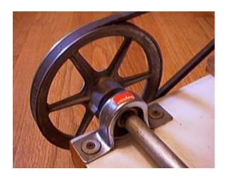
The drive shaft for the mill is 5/8 inch round steel bar stock. These can be purchased at any hardware store. Be sure it is perfectly straight. The sheave on the drive shaft is a 6 inch o.d. by 5/8 inch (Grainger #3X919). This cost me \$3.72. You will also need two selfcentering ball-bearing pillow-block bearings to mount the drive shaft (Grainger #2X898). I had to sand the drive shaft a little bit to allow the bearings to slide onto the shaft.
