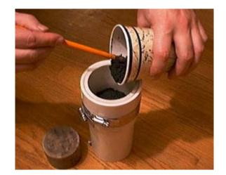
milling time. I would be remiss if I didn't mention that the milling should be done with all the due precautions taken. This means locating the mill remotely and perhaps using protective barriers around it.
