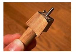
The last part of the tool set is the crossette insert. I started by marking the face of a 1 inch hardwood dowel as shown. The arcs are drawn with the aid of another piece of 1 inch diameter dowel. A hole is drilled in the center to accommodate the insertion of a tapered pin later. A length of 11/16 inch of the drilled dowel is cut from the end.
