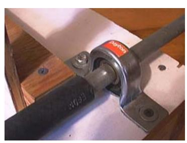
Before placing the bearings on the shaft, you need to place a piece of automotive heater hose on it as shown here. This hose is 5/8 inch i.d. by 7/8 inch o.d. It can be found at most hardware or auto parts stores. A little lubrication of some kind on the shaft will greatly aid the sliding on of the hose.
