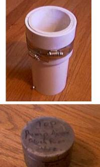
When placed on the base, the compression sleeves form the walls of the chamber where black powder meal is placed to be pressed.
