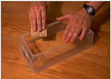
Before applying the epoxy, you should rough up the gluing surface of the plastic with some coarse sand paper.
