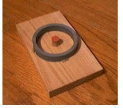
First, we need to gather materials to use for the base and sleeves in the tooling set. I used a piece of oak with dimensions of 3.5" X 6" X 5/8". The sleeves are cut from a piece of 2.5 inch schedule 40 PVC conduit pipe. One is a 1/2 inch slice and the other is 2.5 inches long. Each piece of conduit has been cut along its length by using a coping saw with a very narrow kerf.
