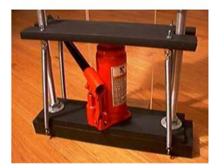
This view from the opposite side of the blast shield illustrates the attachment and placement of the retraction springs. The springs add stability to the middle pressing deck and conveniently retract it when the release valve of the jack is opened. These springs are fairly expensive at \$2.85 apiece, but are well worth the contributions they make to the design.
