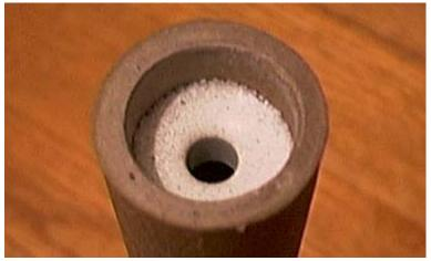
Before I started using the epoxy fillet, the sharp edge of the nozzle throat would usually crumble in a few places as the spindle tooling was extracted. Now, as shown in this picture, the nozzle throat comes out perfect every time. Your fountain nozzles will be the envy of all your pyro buddies.
