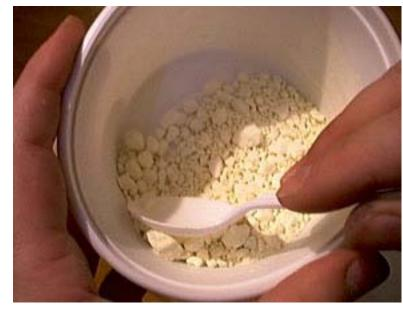
mixture through a 40 mesh screen, many large lumps of sulfur are revealed. These lumps obviously destroy the homogeneity of the mix in their near vicinity.
