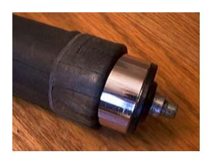
The other side of the mill jar cradle uses a ball bearing equipment roller. I bought this one at Woodworker's Warehouse for about \$10. This picture shows the roller removed from its bracket. The roller has been covered with two layers of bicycle tire inner tube. The inner tube layers have been folded back in the picture for illustrative purposes only. You may be wondering how to get the inner tube layers over the roller. Again, Lloyd describes a
