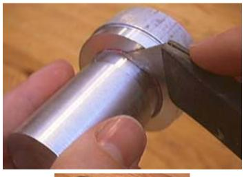
After the rammer has been pressed into the former, I use a utility knife to trim off the ragged edges. Because the cardboard has been moistened, it cuts fairly easily by rocking the knife edge against the rammer. The result, after drying for a few hours, is a very neat looking and strong end cap.
