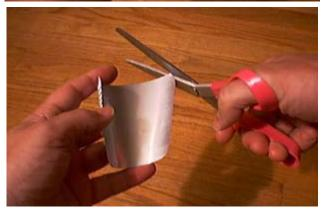
I usually rough cut the shapes with the scissors and then straighten all the edges with a desk top paper cutter. Finally, you will want to use the scissors to round off the sharp corners.
