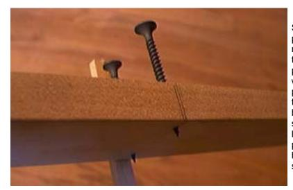
Some careful precision is needed to ensure that the screws are placed on a line which is perpendicular to the line of the beam. I used a Tsquare to draw the line and a drill press to drill guide holes for the screws.
