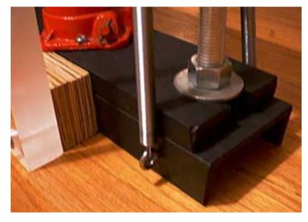
the press is assembled identically to the top. The retraction springs are attached to eye bolts which are mounted through the base channel.
