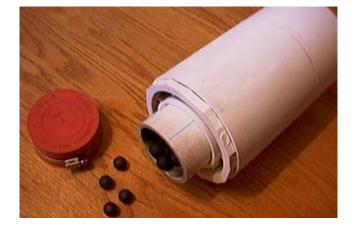
This is a mill jar which has been constructed from 5 inch PVC pipe and fittings. The milling media is antimony hardened, 3/4 inch lead balls. The construction of the jars is relatively simple, but is a subject for another project page.
