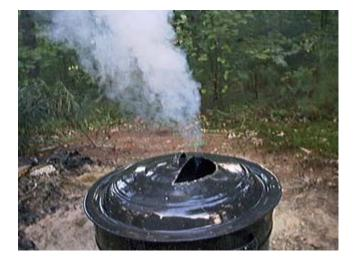
OK, we've finished making our primo charcoal cooker. Let's talk about how to use this hi tech apparatus. Perhaps the most labor intensive part of making charcoal is the preparation of the wood. When using willow, you must remove the bark and split the sticks into smaller sticks no thicker than 1/2 inch. I load the retort as full as possible with the sticks oriented vertically.
