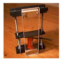
Finally, the finished product is shown. This press design was partially inspired by a similar plan sold by Firefox Enterprises. The major difference is that the Firefox design places the hydraulic jack on top of the pressing deck and the object to be pressed is placed on the base of the pressing frame. This way, the pressing surface comes down from above, whereas the design shown here causes the pressing surface to push up. If you are interested in the Firefox design, it only costs \$4.00.
