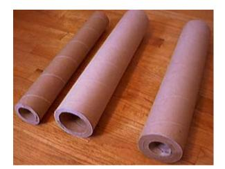
The original description of this project calls for a paper tube with a 4 inch outside diameter, 2 inch inside diameter and 1 inch thick walls. This is required because of the tremendous pressures that must be withstood by the fountain. Until recently. this kind of paper tube could not be purchased, but you can now get them from Dawntreader Pyrotechnic Specialties. It is made by bonding one tube inside another to achieve the total wall
