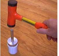
Because of the amount of compression in the cardboard, it is very difficult to extract the rammer from the former. I use a short piece of 2 inch PVC and a dowel pin, as shown here, to gently tap the rammer and finished end cap out of the former.
