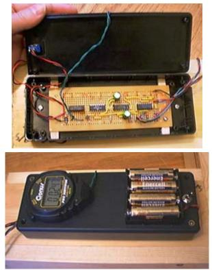
This picture shows the circuit board mounted in the enclosure box . A Radio Shack (cat. no. 276-170) proto board and project box (cat. no. 270-1808) were used at a cost of about \$6 US for both. A battery pack with four AA batteries is mounted on the outside of the enclosure for easy access.
