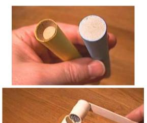
An end plug can be made by ramming about 1/2 inch of bentonite clay into the bottom of the tube. A better alternative is a paper end plug from Skylighter (item #198), but the drawback is that you have to buy 500 of them at a time. That would be enough to last me about 49 years. I suppose you could make your own paper end plug, but I'm too lazy to even consider that option.
