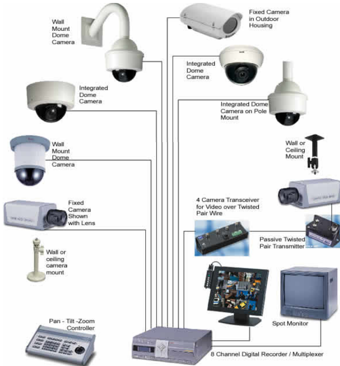
Figure 1.2. Overview of CCTV equipment and system design 45
