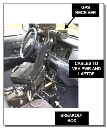
Figure 2. In-Vehicle Configuration of GPS Receiver
