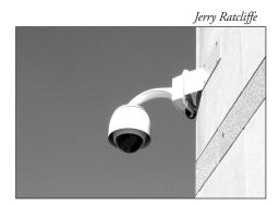
This semi-covert CCTV camera may have a crime prevention advantage over an overt system because offenders can never be sure in which direction that camera is facing.
