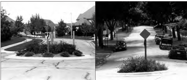
Traffic circles, of varying sizes, reduce speeds and crashes in residential areas.
