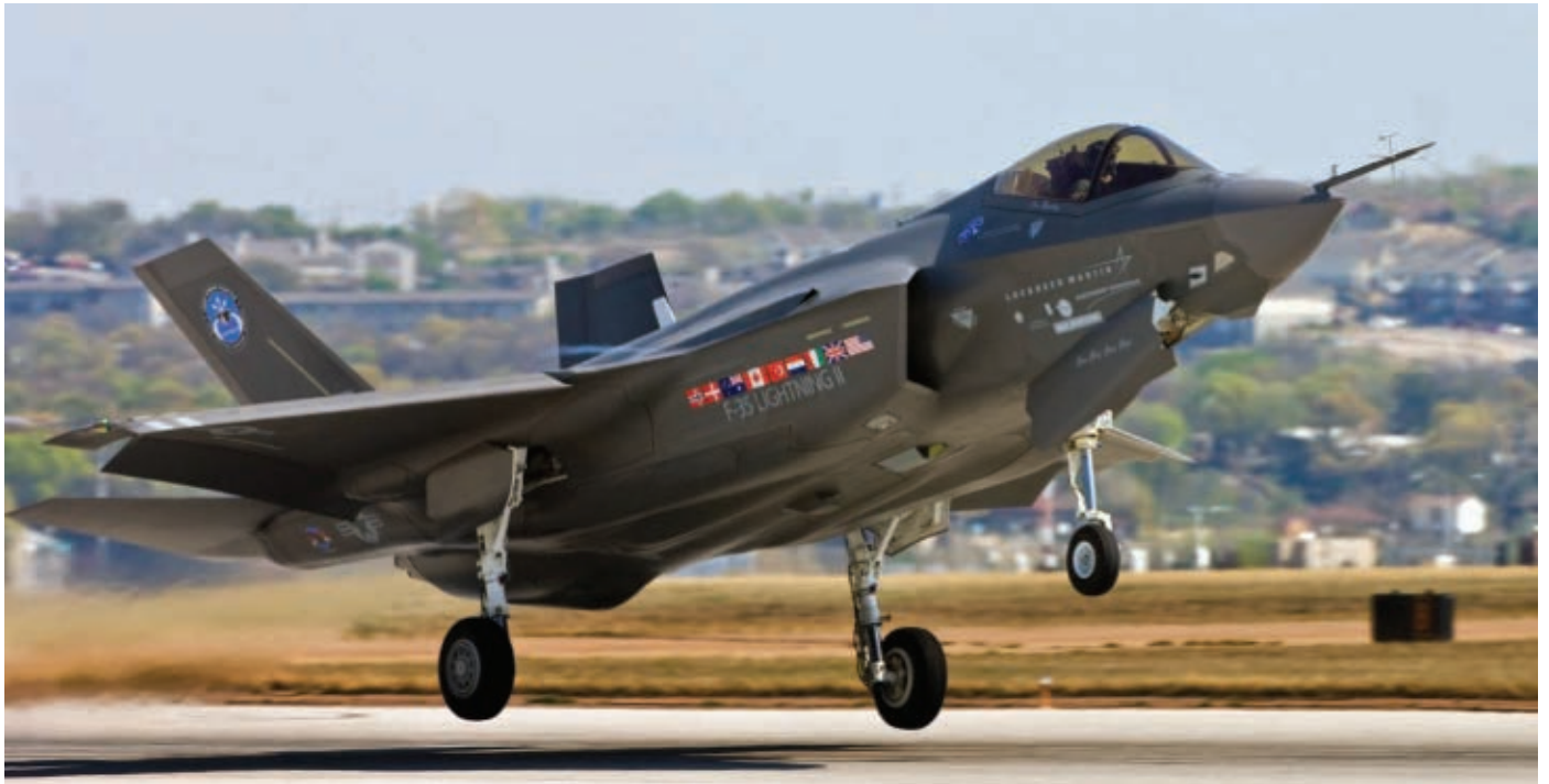
The F-35 is a multirole, stealth-capable supersonic aircraft. The Marine version will be short takeoff and vertical landing capable. (Photo by John E. Wilson, Lockheed Martin.)
