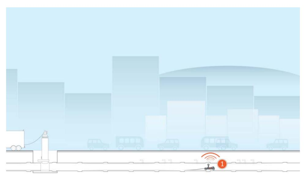
1. Visually Identify Path of Main or Feature: ULC Operator positions sonde-enabled VGC robot, patented PRX250 camera or CISBOT robot below pipeline feature
