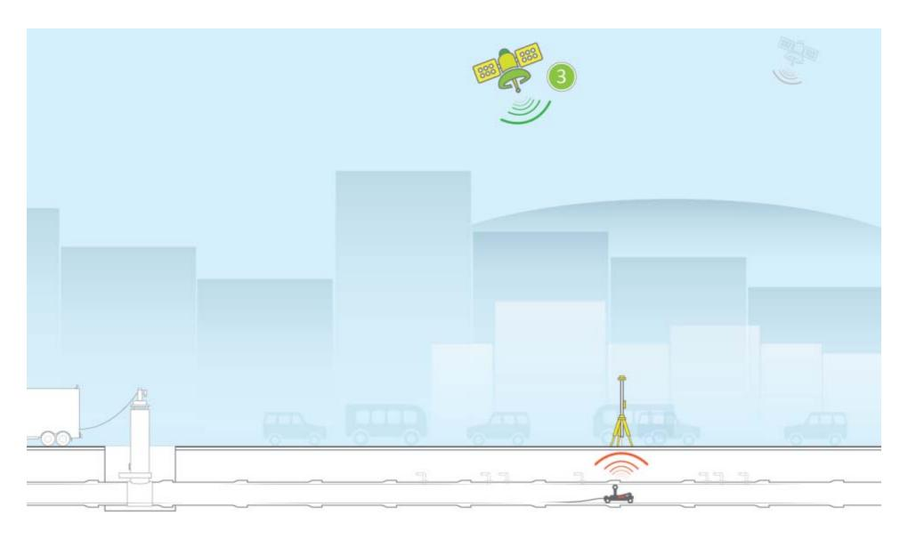
**3. Obtain GPS Location:** GPS tripod communicates directly with satellites and reference stations to obtain 1-2cm accurate GPS location.
