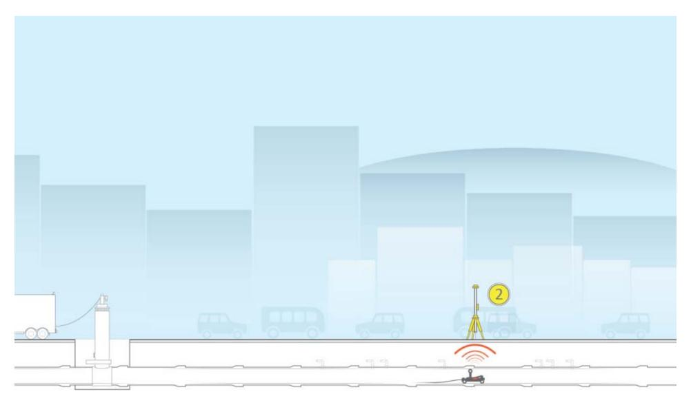
2. Technician positions tripod: ULC Technician positions the tripod directly over the locate point using an integrated laser to ensure accurate positioning.
