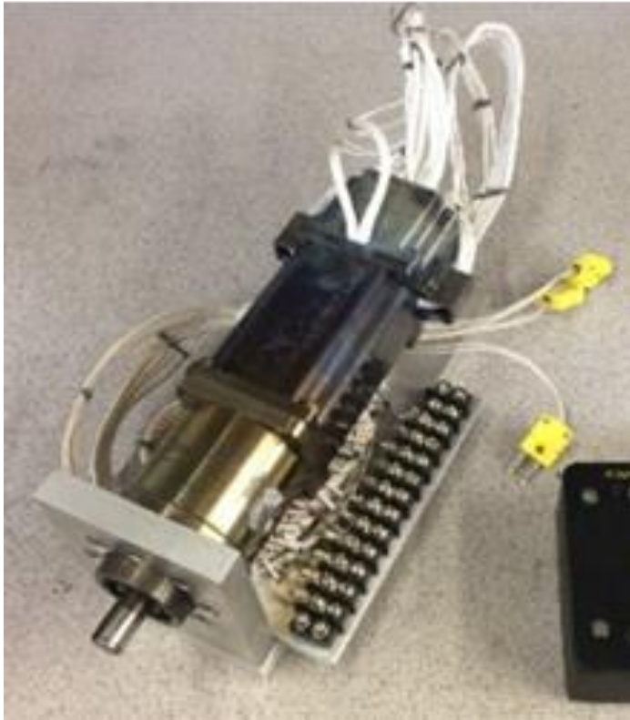
Actuator: Planetary gearbox, BLDC Motor, PIPS sensor
