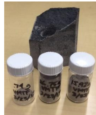
Simulant fines generated by the drill
