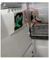
②As shown in the figure, pull out the two terminals those are connected to the freezer air duct; roll out the freezer air duct from below. There are two connection terminals, which are the freezing fan and the freezing sensor.
