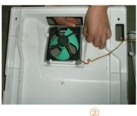
② Take the fan cable out. Unscrew three bolts with a cross screwdriver. Disassemble the freezer fan.
