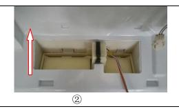
② Follow the arrow direction in the figure and slightly pull out the refrigerator air door from top to bottom.
