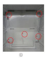
①Unscrew five bolts from the freezer air duct with a cross screwdriver;
