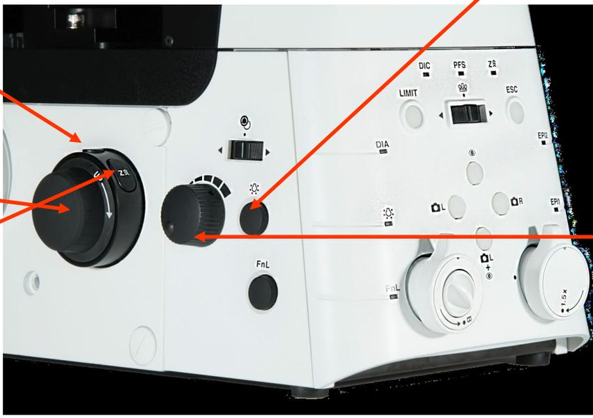
DIA brightness adjuster: adjusts the brightness of the diascopeic lamp
