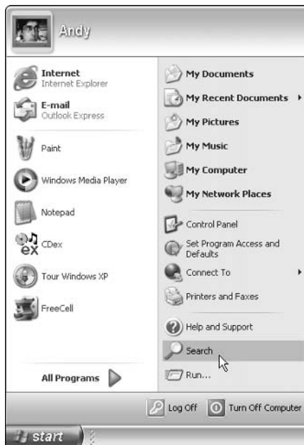
Figure 6-2: Click the Start button and choose Search to look for things on your computer or the Internet.
