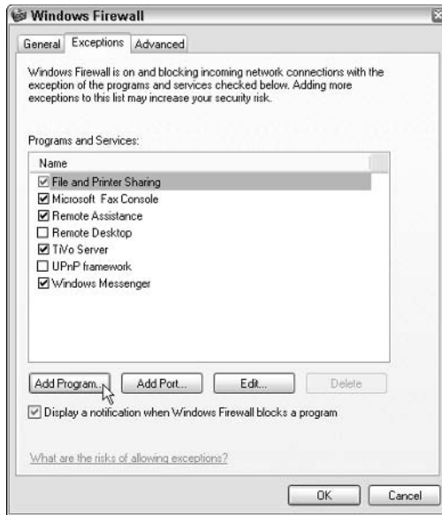
Figure 10-2: If the firewall blocks a program unnecessarily, add the program to the exceptions list.
