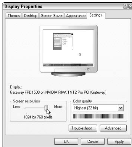
Figure 11-5: Depending on the screen resolution, Windows can squeeze different amounts of information onto your monitor.
