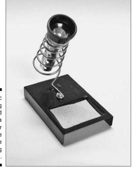
Figure 16-2: A soldering stand provides a holder for the sponge and the soldering iron.
