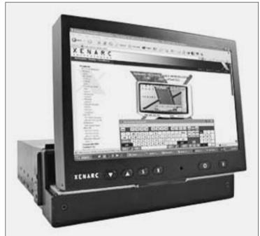
Figure 14-2: A Xenarc Model 700IDT for in-dash DIN mounting.
