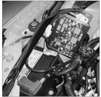
Figure 13-3: A close-up of the battery and the fuse box with its cover removed.
