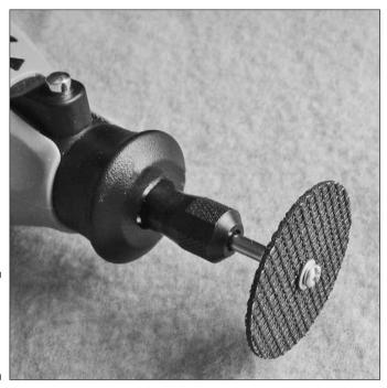
Figure 16-6: A cutting blade on a hand-held Dremel.
