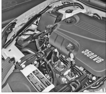
Figure 13-2: The fuse box is the black square box near the top in the Chevy Impala.
