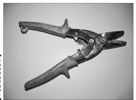
Figure 16-7: My trusty old tin snips are great for cutting the metal shielding inside computers.
