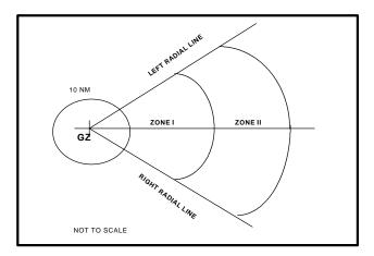
4.3.5. Step 4. Draw two tangent lines from the cloud radius circle to the points of intersection of the left and right radial lines with the Zone I arc. Time of arrival arcs are entered on the prediction using dashed lines (see Figure 4.6.). To determine time of arrival at a specific point, use the formula:
