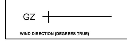
4.3.3. Step 2. Draw two radial lines from GZ; one 20 degrees to the right, the other 20 degrees to the left of the downwind distance (see Figure 4.4.).
