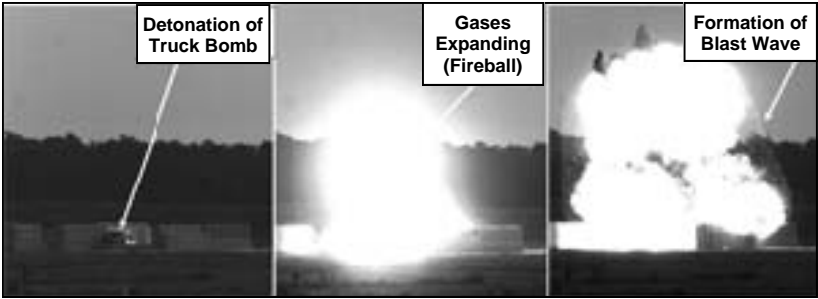
Figure 11-2. High-speed camera sequence showing blast wave formation
