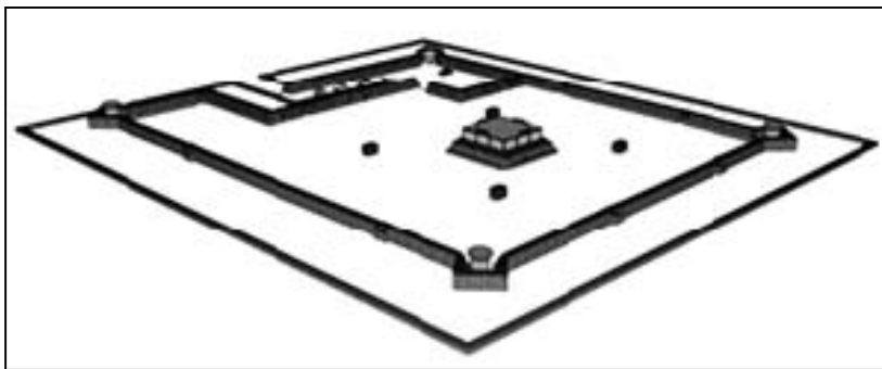
Figure 21-4. Double-wall perimeter system concept
