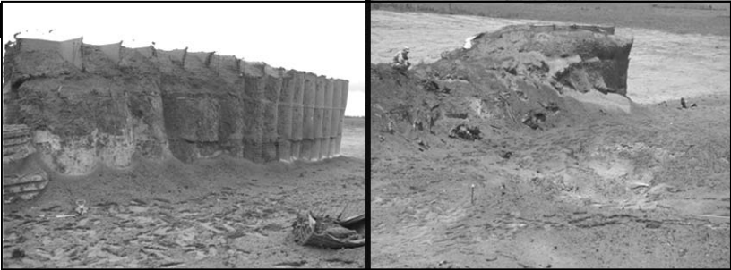
Figure 21-15. Second explosion test of inner wall (Left: Before; Right: After)
