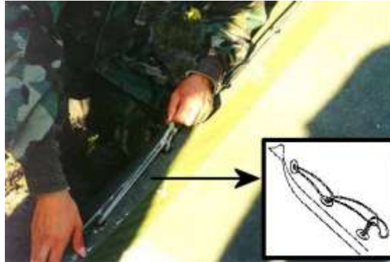
Figure 3.20. Closing of Hook and Pile Fastener Weather Flap.
