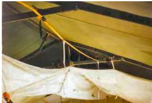
Figure 3.36. Light Support Strap Assemblies.
