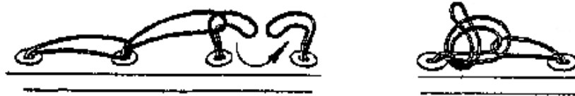
Figure 3.21. Tying Half-Hitch Knot in Last Lace at Eave.
