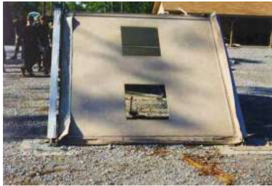
Figure 6.15. Breached Panel Section.
