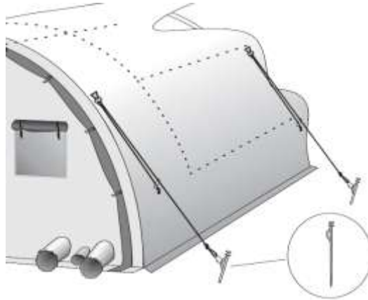
Figure 2.20. Guy Rope Installation.
