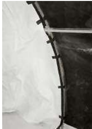
Figure 2.28. Remaining Fasteners Attached to Center Arch.
