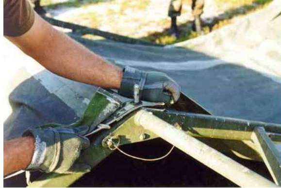
Figure 3.18. Large Grommet Placed Over Ridge Joint Spindle.
