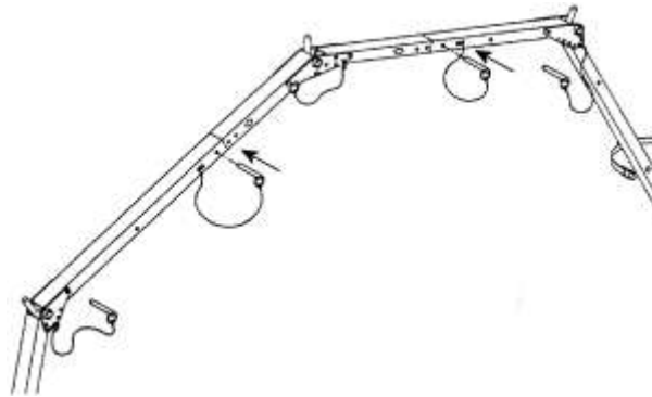
Figure 3.12. Connecting Roof and Side Arch Assemblies.
