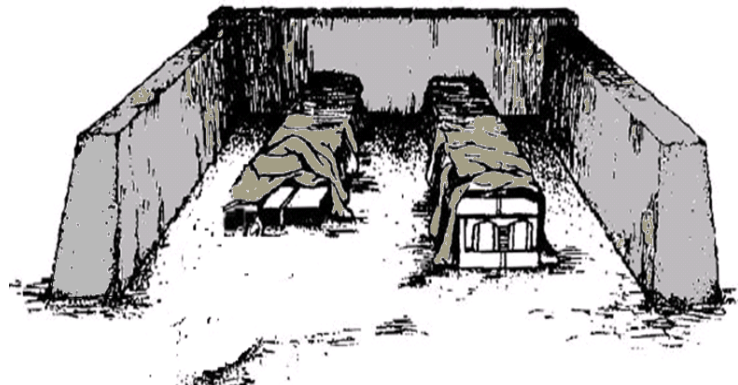
Figure 5.20. Soil-Cement Revetment.
