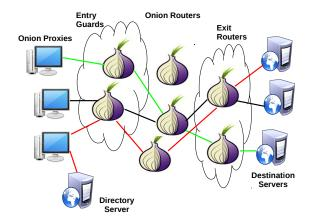
Fig. 1. The Tor Network: Clients (running OPs) contact the directory servers periodically to get a list of ORs and their descriptors. Clients then use Tor's router selection algorithm to build circuits. A circuit consists of three hops: entry guard, middle and exit. The exit performs the TCP connection on behalf of the user to the user's destination.
