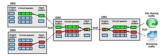
Fig. 2. This figure (adapted from AlSabah and Goldberg [2013]) shows Tor's application-level queueing architecture. Tor maintains input buffers, circuit queues, and output buffers, in addition to the kernel's TCP buffers. This figure also demonstrates the cross-circuit interference problem (see Section 3.5).
