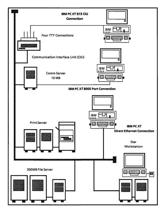
Fig. 1. Typical XNS Ethernet Environment Illustrating the Three Types of Connections for the IBM PC XT
