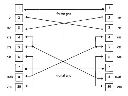
Fig. 2. Asynchronous Modem Eliminator
