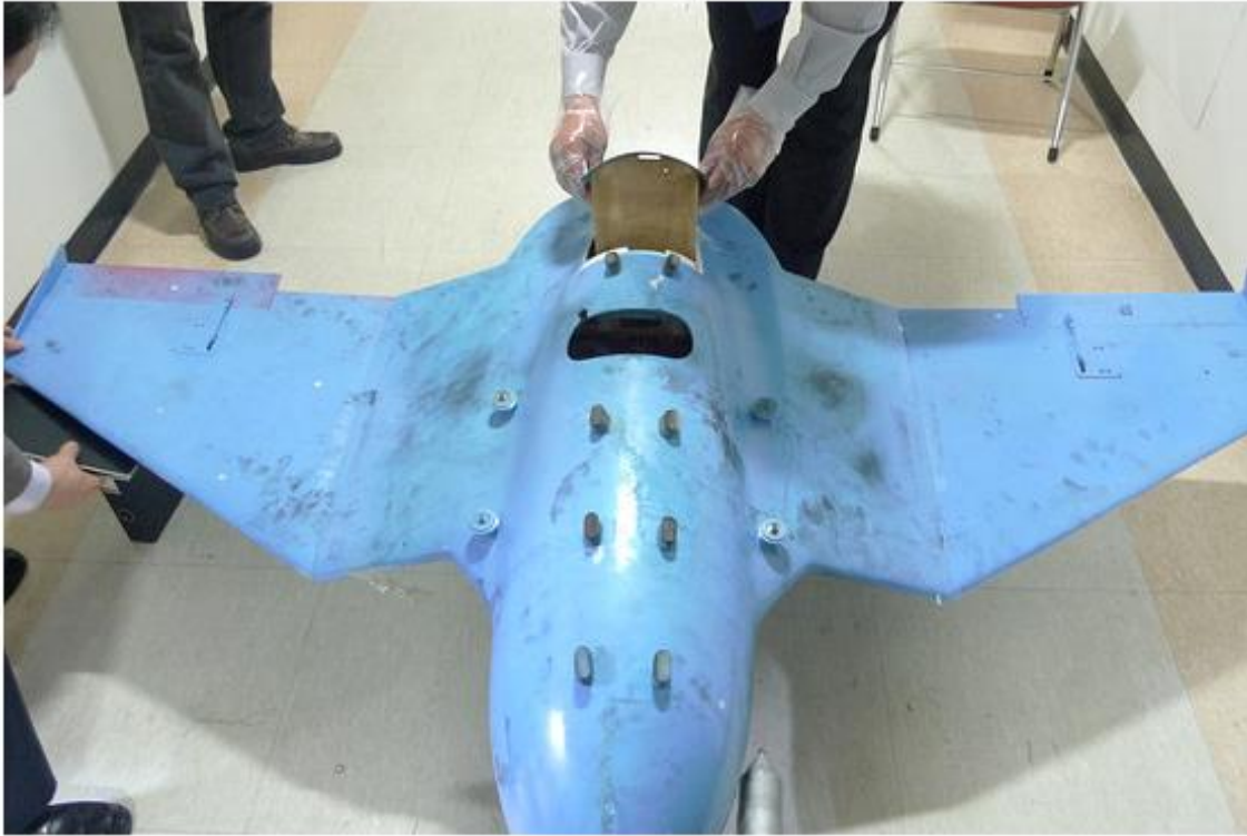
The underside of the drone found in Paju, with a hole that appears to allow photos to be taken of the ground area. — South Korea's Ministry of Defense
