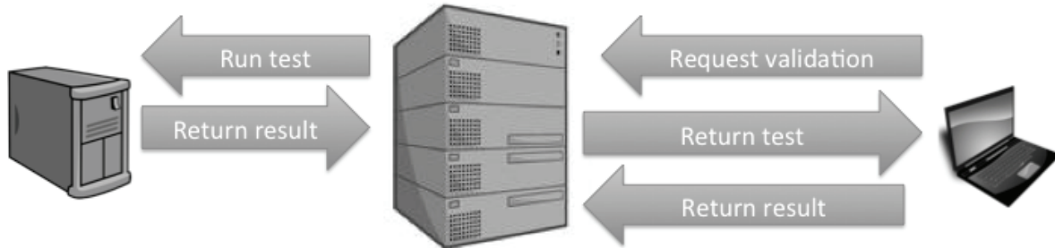
Figure 3: Naïve verification procedure. The remote machine (on the right) requests validation. The distributor (in the middle) generates a test and runs it on a local machine (on the left). The local machine returns the result to the distributor. The distributor sends the same test to the remote machine. The remote machine runs the test and returns the result to the distributor. The distributor compares the results received from the local and remote machines. If the results are equal the validation succeeded
