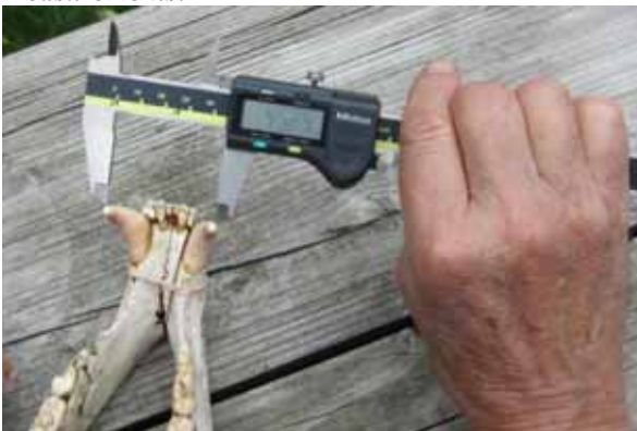
Figure 3: NJ-BB-030. Measuring the mandibular canine cusp tip. Intercanine width as measured at the canine cusp tips. Measurement 45.29mm + 1.30mm saw cut width. Intercanine width = 4.659cm. This measurement is appropriate for shallow or superficial bites.
