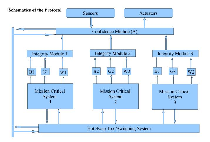
Figure Y : Schematics of the Protocol
