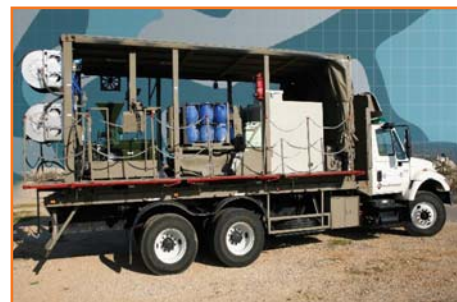
Girit – NBC Decontamination Unit to be mounted on truck when needed, equipped with unique mixer device to perform thorough area decontamination
