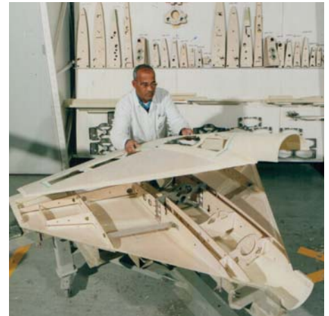
Harpy Loitering Attack UAV Composite Fuselage Construction
