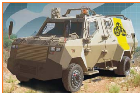
Sniffer – NBC Reconnaissance Armored vehicle equipped to meet customer's demands for Detection & Identification of Hazardous NBC agents
