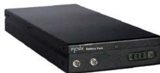
Internal 1U size battery pack to support 5 - 7 hours of Passive system
