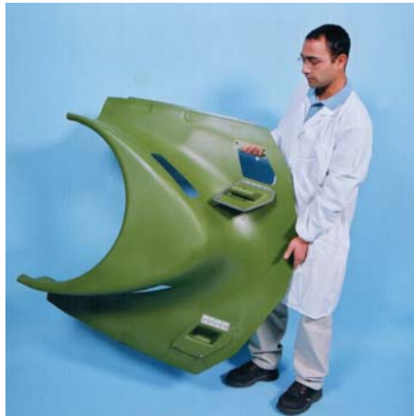
Light-Weight Composite Helicopter Structure
