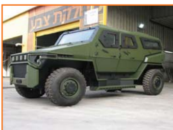
Hurricane – An 8 Ton all terrain 4X4 APC, up to 7 people, KE Stanag 2 and Mine protection Stanag 3a+2b
